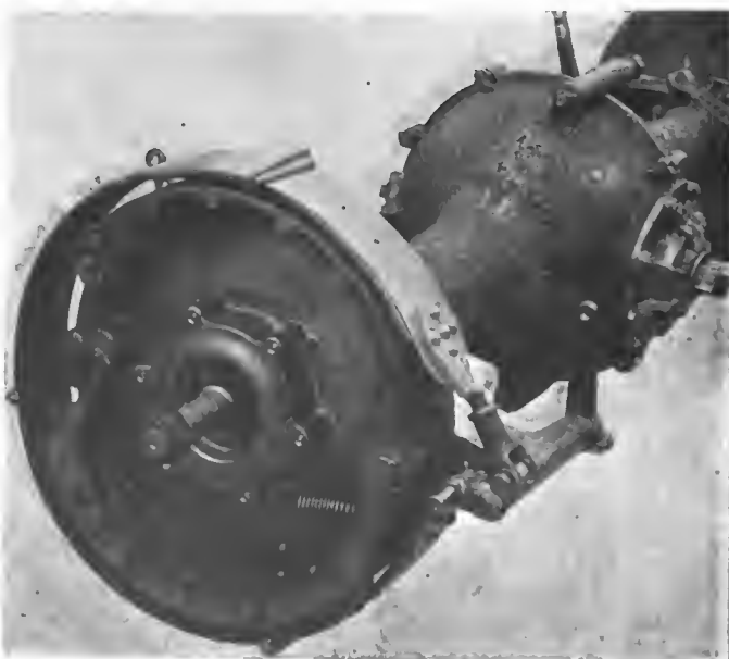
BRAKE DRUM ASSEMBLY SHOWING LARGE NUMBER OF CORK INSERTS.
